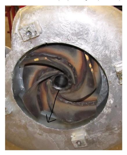
Refit the impeller and assemble the pump by following instructions in reverse order.
