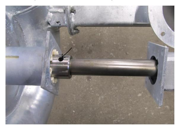
Remove the cutter on the pump housing and pull the impeller out of the pump housing.
