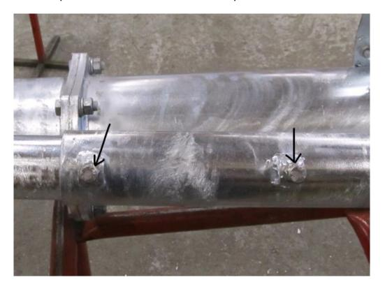
Unscrew the four screws that secure the cover tube to the pump housing.
