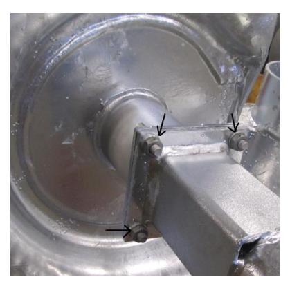
Detach the cover tube from the pump housing and push it upwards that the shaft will be seen. Push out the cotter pin which secures the shaft to the impeller.
